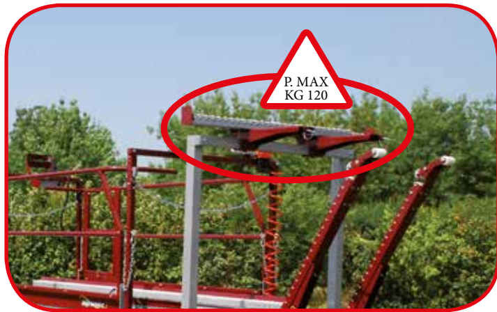
SUPPORTO SUPPLEMENTARE BINS APPLICABILE SIA ANTERIORMENTE CHE POSTERIORMENTE ADDITIONAL BINS SUPPORT FRONT/BACK MOUNTABLE ZUSÄTZLICHE KISTENUNTERSTÜTZUNG VORNE/RÜCK SUPPORT BINS SUPPLEMENTAIRES AVANT/ARRIERE SUPORTE ADICIONAL BINS MONTABLE DELANTERO/TRASERO
